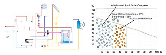
This combination is a new highlight in relation to technique and esthetics. Solar COMPLEET increases the COP per year of an air/water heat pump > 4 and the solar output by 25% in respect to conventional systems. This is an investment into the future that amortizes after a few years.
