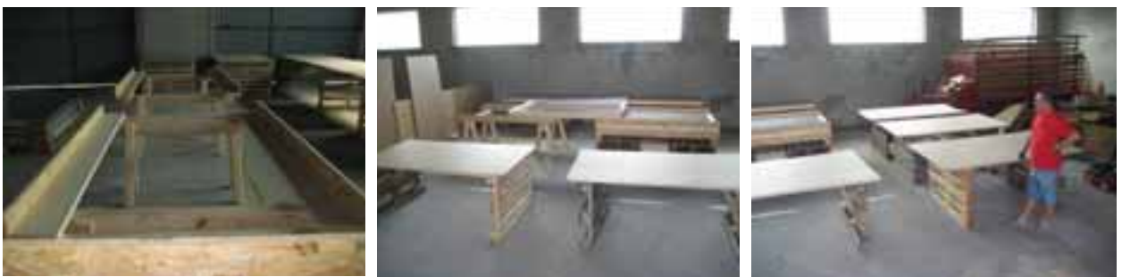
1:1 model made of wood / carton to analyse the working steps of the production
