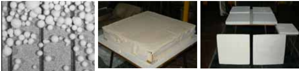
Fig. 2. Microscope photo of PCM capsules and PCM based plasterboards
