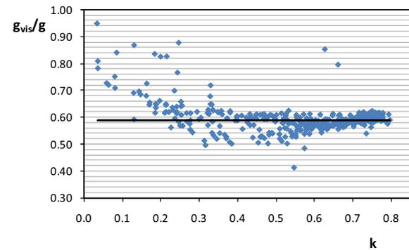
Figure 18. Clear glass. Hourly values of the fraction in the visible band  $g_{vis}/g$  in relation to clearness index  $k$  for July.
