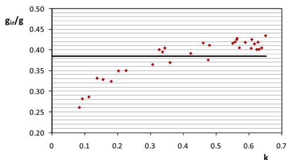
Figure 5. Clear glass. Daily values of the fraction in the infrared band  $g_{ir}/g$  in relation to clearness index  $k$  for January.
