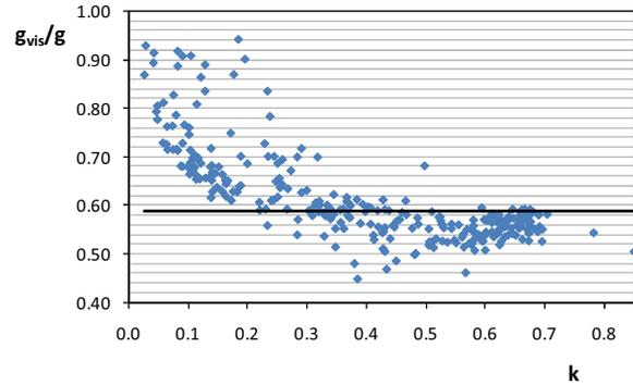
Figure 16. Clear glass. Hourly values of the fraction in the visible band  $g_{vis}/g$  in relation to clearness index  $k$  for January.
