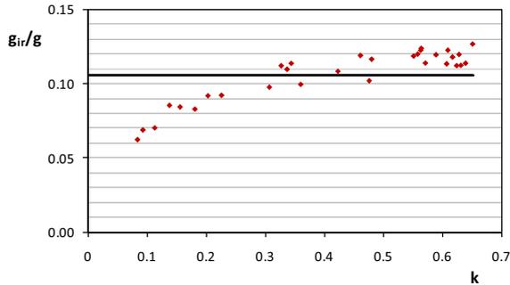
Figure 9. Selective glass. Daily values of the fraction in the infrared band  $g_{ir}/g$  in relation to clearness index  $k$  for July.
