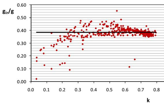
Figure 17. Clear glass. Hourly values of the fraction in the infrared band  $g_{ir}/g$  in relation to clearness index  $k$  for July.
