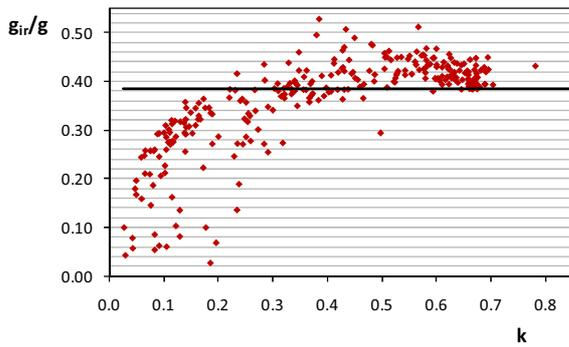
Figure 15. Clear glass. Hourly values of the fraction in the infrared band  $g_{ir}/g$  in relation to clearness index  $k$  for January.
