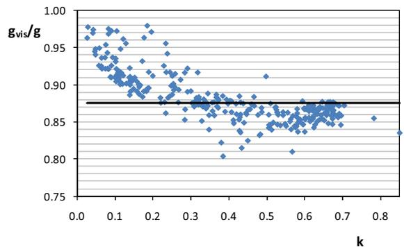
Figure 20. Selective glass. Hourly values of the fraction in the visible band  $g_{vis}/g$  in relation to clearness index  $k$  for January.
