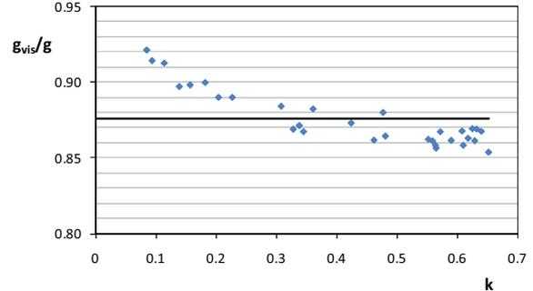
Figure 10. Selective glass. Daily values of the fraction in the visible band  $g_{vis}/g$  in relation to clearness index  $k$  for July.
