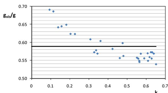
Figure 6. Clear glass. Daily values of the fraction in the visible band  $g_{vis}/g$  in relation to clearness index  $k$  for January.
