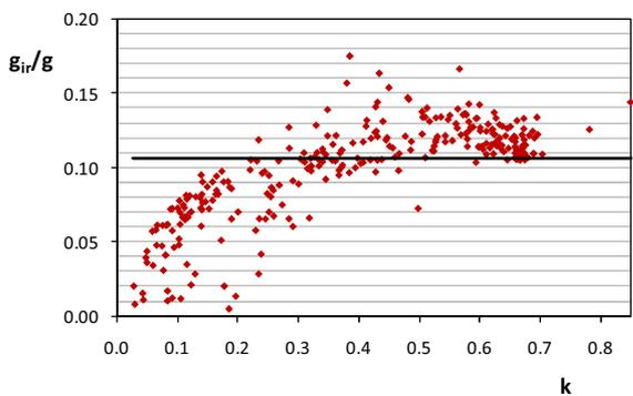
Figure 19. Selective glass. Hourly values of the fraction in the infrared band  $g_{ir}/g$  in relation to clearness index  $k$  for January.
