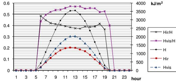
Figure 1. Hourly trend of global solar radiation H, visible  $H_{vis}$  and infrared  $H_{ir}$ , and fractions of the solar spectrum contained in the two bands  $H_{vis}/H$  and  $H_{ir}/H$ . Clearness index  $k=0.733$ .
