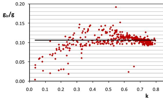
Figure 21. Selective glass. Hourly values of the fraction in the infrared band  $g_{ir}/g$  in relation to clearness index  $k$  for July.
