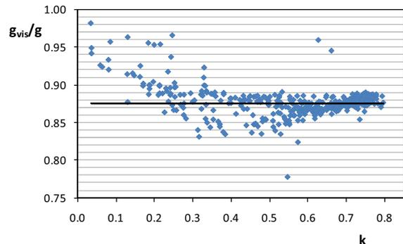
Figure 22. Selective glass. Hourly values of the fraction in the visible band  $g_{vis}/g$  in relation to clearness index  $k$  for July.
