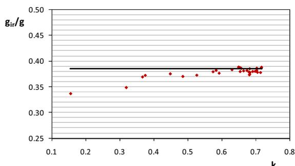
Figure 7. Clear glass. Daily values of the fraction in the infrared band  $g_{ir}/g$  in relation to clearness index  $k$  for July.
