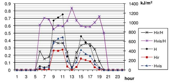
Figure 2. Hourly trend of global solar radiation H, visible  $H_{vis}$  and infrared  $H_{ir}$ , and fractions of the solar spectrum contained in the two bands  $H_{vis}/H$  and  $H_{ir}/H$ . Clearness index  $k=0.155$ .
