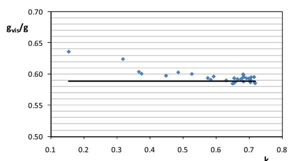
Figure 8. Clear glass. Daily values of the fraction in the visible band  $g_{vis}/g$  in relation to clearness index  $k$  for July.
