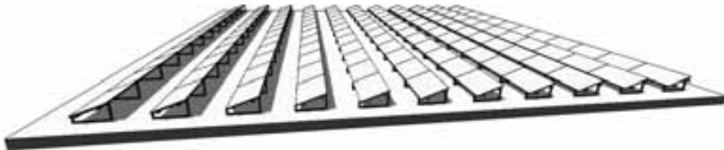
Fig. 1. Typical layout of a roof-top PV plant with the modules mounted horizontally.
