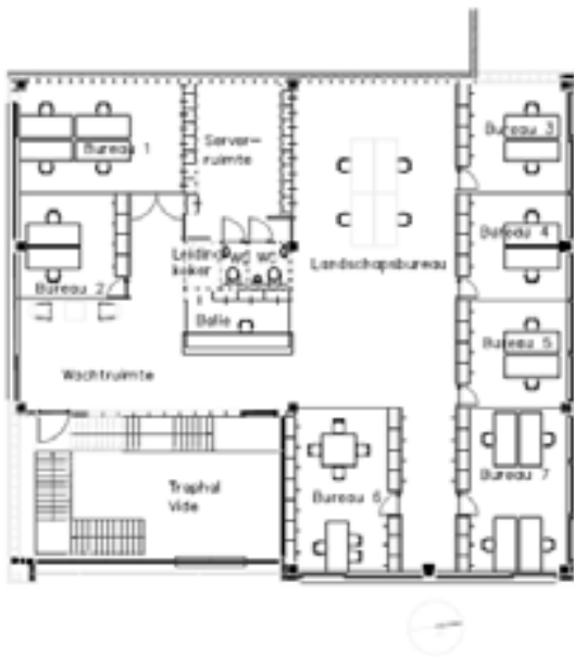
Fig. 1. Office spaces on the first floor.
