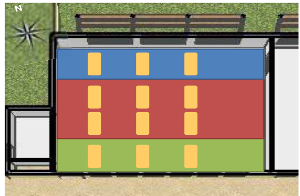
Fig. 7. Daylighting measurements showed that three parallel areas can be defined: the daylighting is very good near the windows overlooking the exterior (blue), slightly weaker in the middle (red) and even weaker on the side of the windows overlooking the other part of the building (green)
