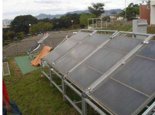
(b) Dirty collectors in the end of the exposition test (05/15/2009)
