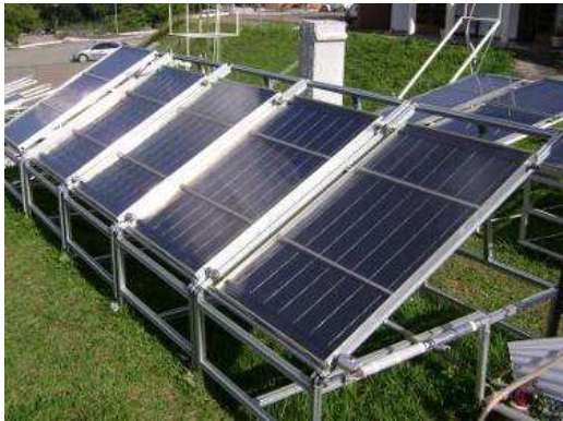
(a) Clean collectors in the beginning of the exposition test (12/10/2008)
