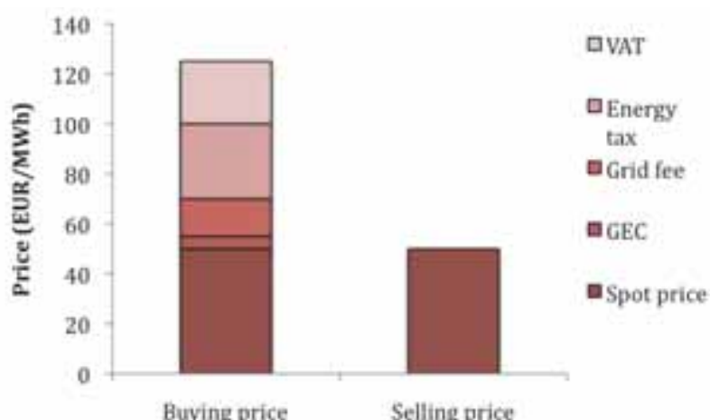
Fig. 3. Typical composition of electricity buying and selling prices for a Swedish household (VAT = value added tax, GEC = green electricity certificate cost).
