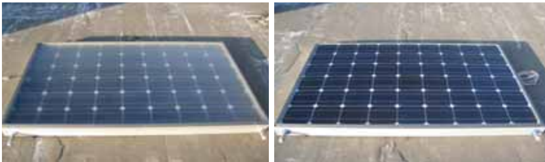
Fig. 3 Tested Glazed and Unglazed PVT collector
