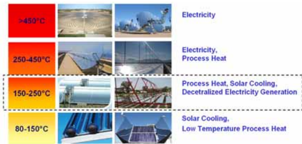
Fig. 1. Overview on concentrating solar collectors. Point focusing collectors are able to generate process heat with temperatures above 450°C. Large Parabolic Troughs and Linear Fresnel Systems are used mainly for large scale electricity generation and use heat transfer fluid temperatures between 250°C and 450°C. Small scale parabolic troughs and Linear Fresnel Systems generate process heat in the range of 150°C-250°C. Low concentrating systems like the new Reflec collector concept are able to generate process heat up to 150°C [4]. Temperature ranges are indicative only.
