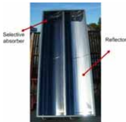
Figure 2 – CPC collector turned 90° during the autumn equinox.
