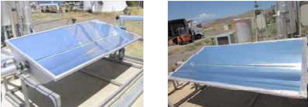
Figure 1. CAPSOL prototypes installed at the PSA: CAPSOL-01 (left) and CAPSOL-02 (right).
