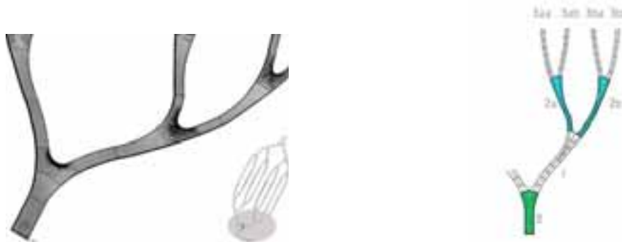
Fig. 8: Part of small absorber (left), nomenclature of branches (right)
