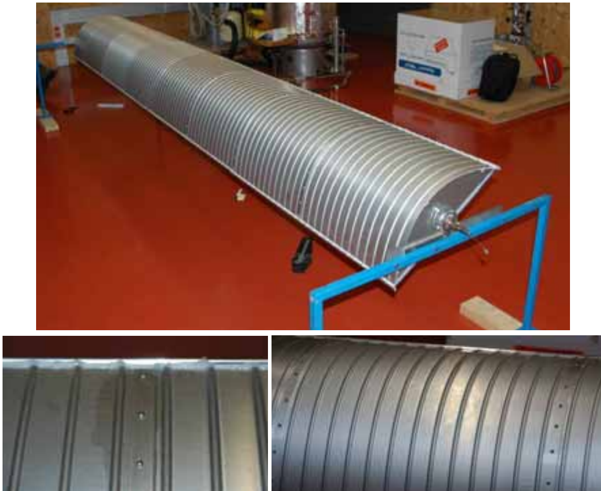
Fig. 1. Collector back made from profiled sheet aluminum.
