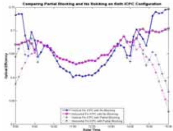
Fig. 16. Partial blocking effects on both vertical Fin and horizontal fin configurations.
