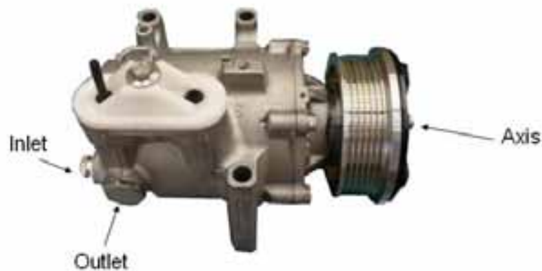
Figure 6. Scroll expander to be characterized in the test bench.
