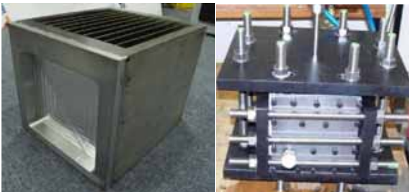
Figure 5: Sorption generator empty and with retaining pressure flanges
