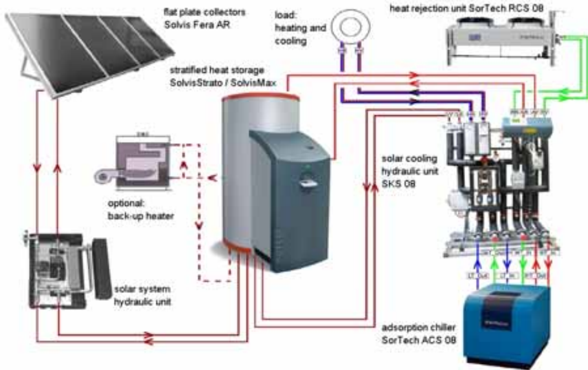
Fig. 1. System schematic: the stratifying buffer storage acts as an energy manager. A pre fabricated hydraulic switching unit distributes hot, cold and chillers fluids to the different components
