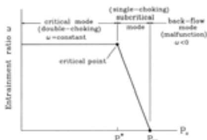
Figure 1 Double-choking phenomenon of ECS.
