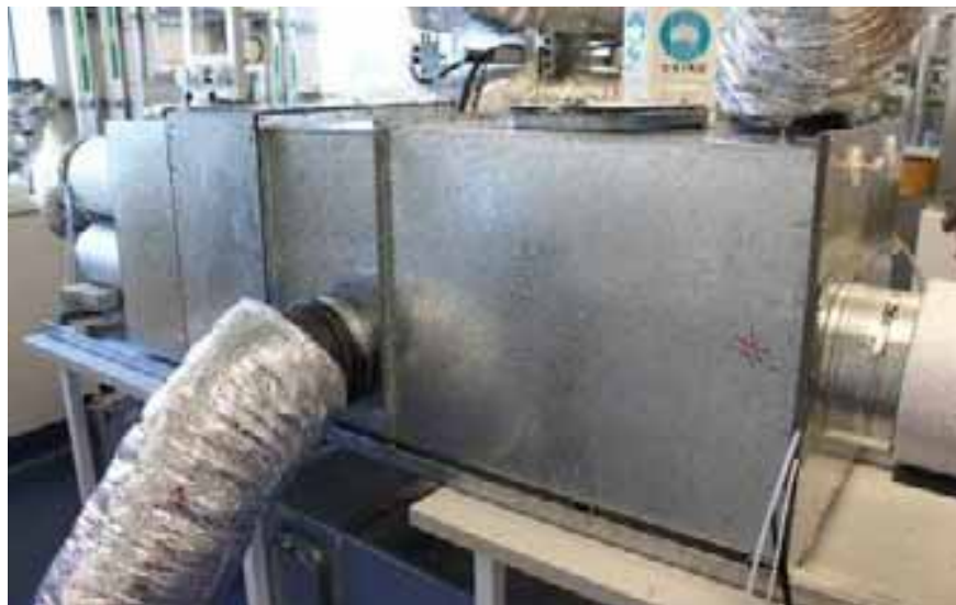
Figure 4: Photograph of the CSIRO-Rinnai Prototype Desiccant Cooler under test in Newcastle.
