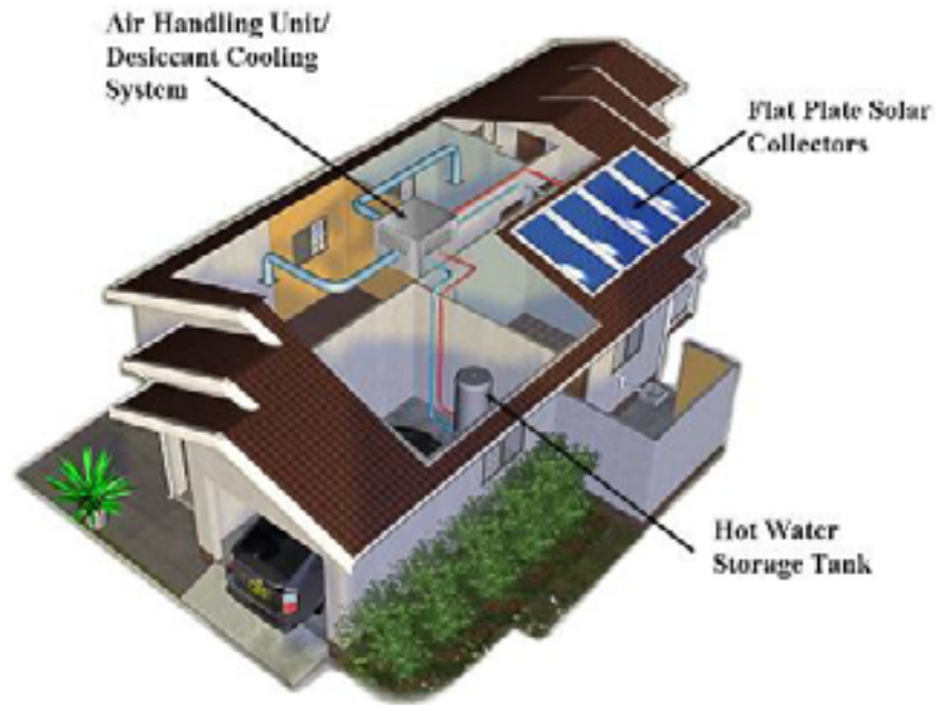
Figure 1: CSIRO and gas appliance supplier Rinnai have developed a new 3-in-1 solar product designed to produce hot water, supply winter space heating; and provide summer space cooling.
