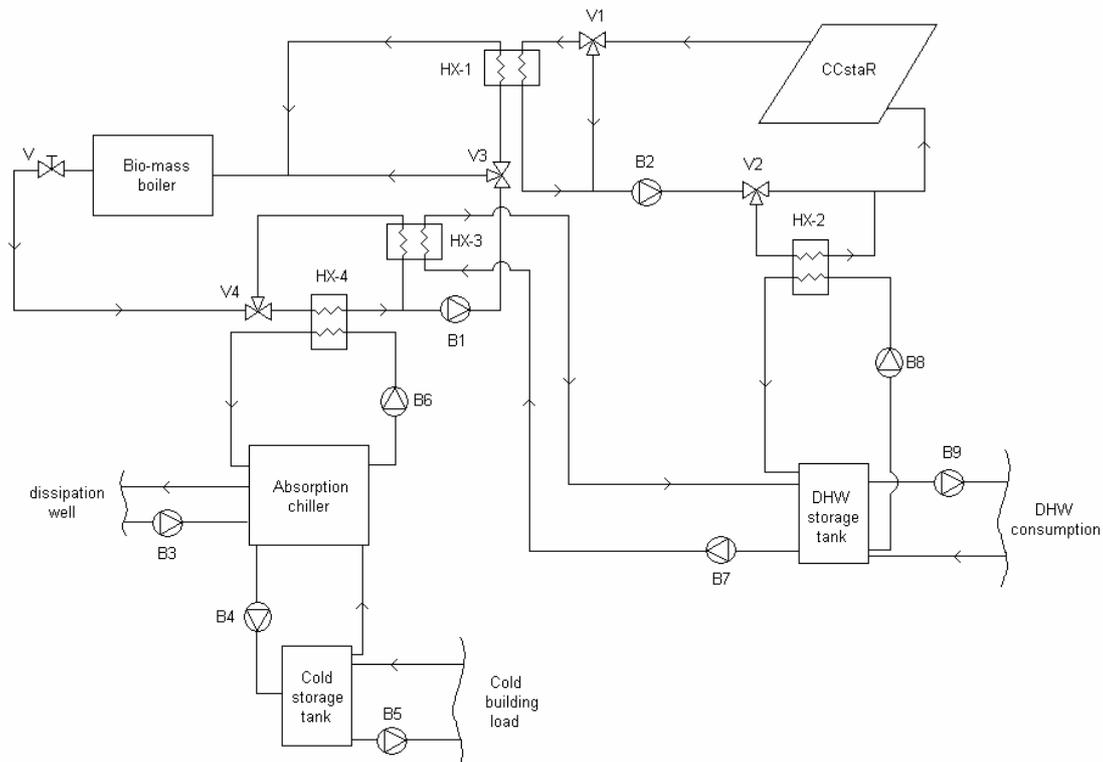
Fig. 1. Process diagram of the solar cooling and DHW system.
