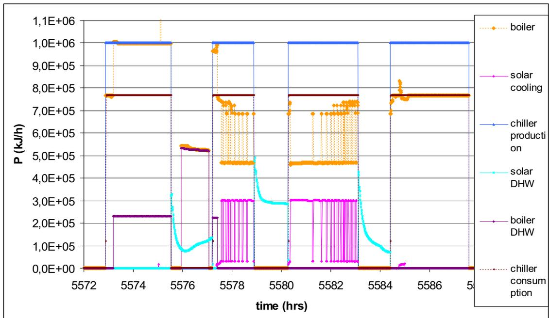
Fig. 3. Simulated system energy rates on 20 August.
