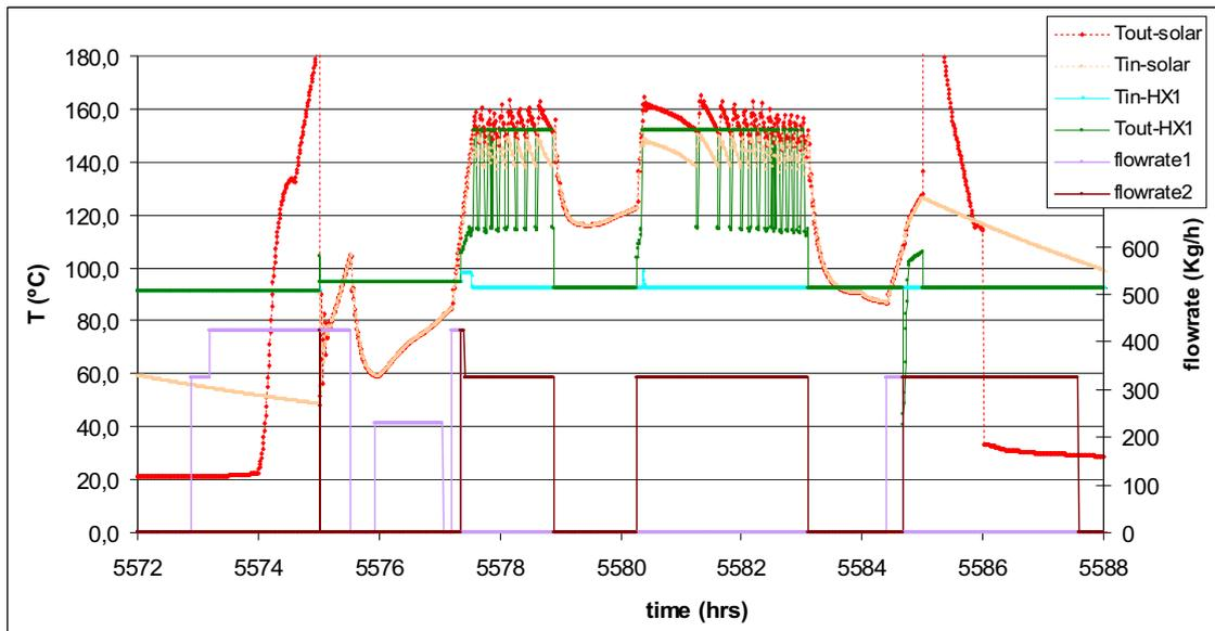
Fig.2. Simulated solar receiver and solar support operation temperatures on 20 August.
