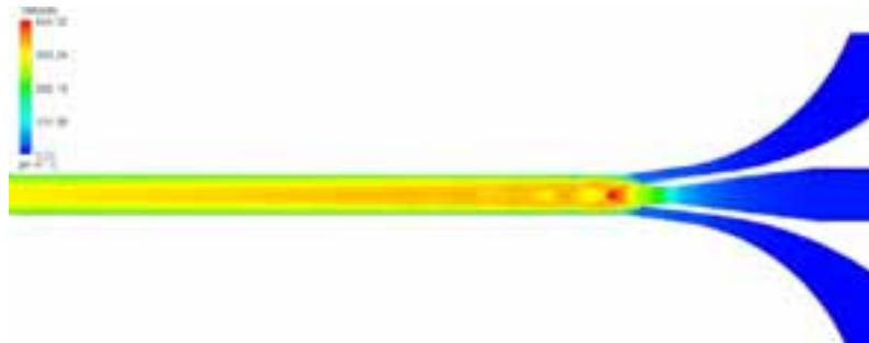
Fig. 1. Velocity profile in the flow part of an ejector ( T_{ev} = 12^\circ\text{C} , T_{con} = 35^\circ\text{C} , T_{gen} = 85^\circ\text{C} ) working with R600a
