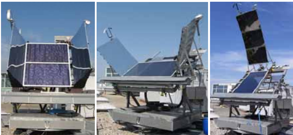
Fig. 1: RefleC test samples during outdoor characterization at the TestLab Solar Thermal of Fraunhofer ISE (efficiency curve position; from left to right: RefleC_1, Oct. 2007; RefleC_2, June 2008; RefleC_3, Aug. 2009)
