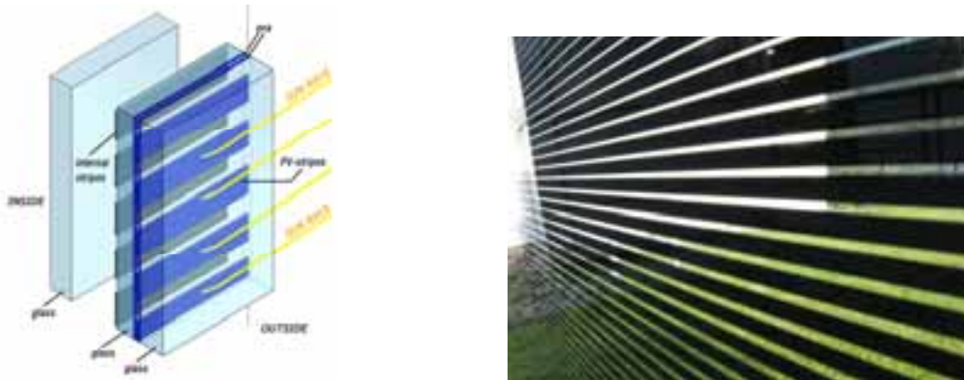
Figure 1: On the left: schematic view of the new see-through, angle-selective façade. The stripes (represented in blue) can be produced with photovoltaic technology. On the right: a detailed view of the first prototype with black ceramic frit stripes is shown.
