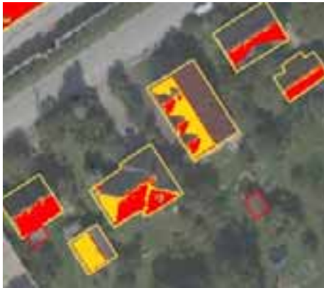
Fig. 8: Suitable solar areas (red roof areas: classified as being very suitable; orange roof areas: classified as being suitable)
