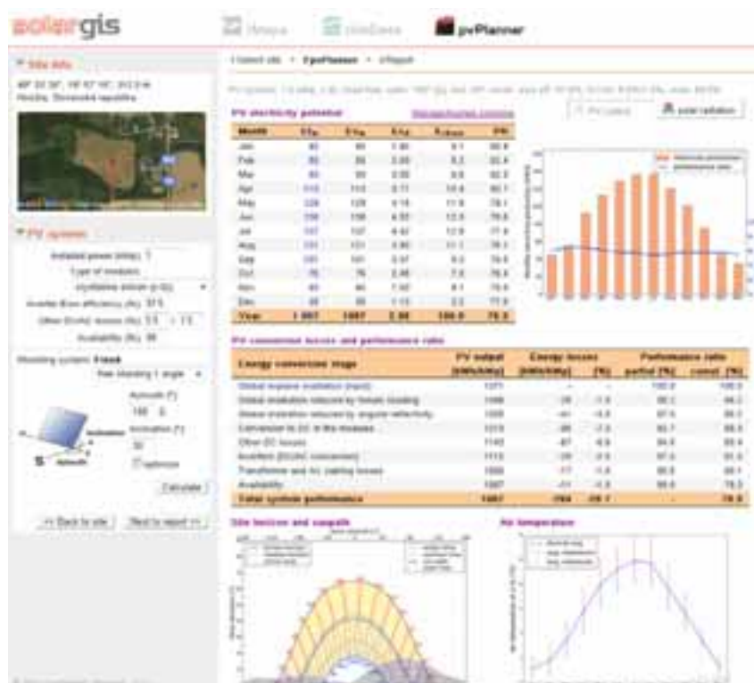
Fig. 4. SolarGIS pvPlanner – simulation of PV electricity potential.
