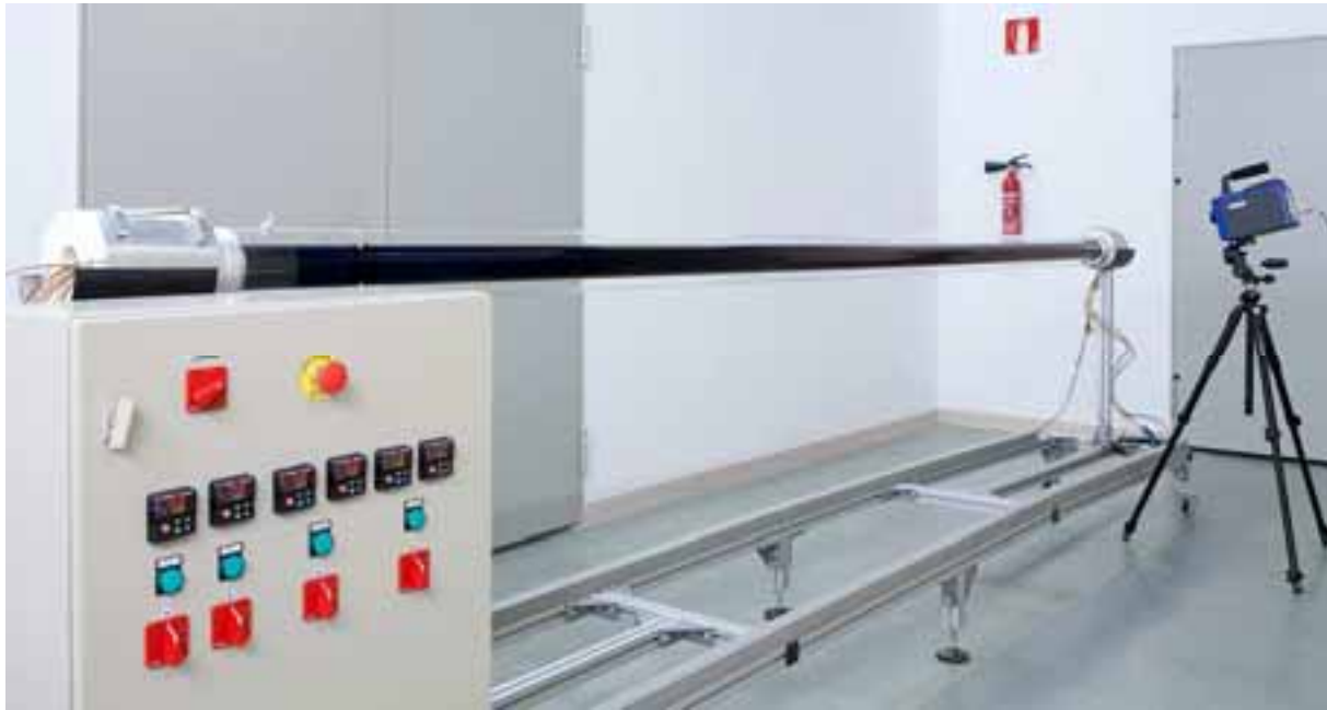
Fig. 2. PTR thermal characterization test bench with IR camera. Source: CENER
