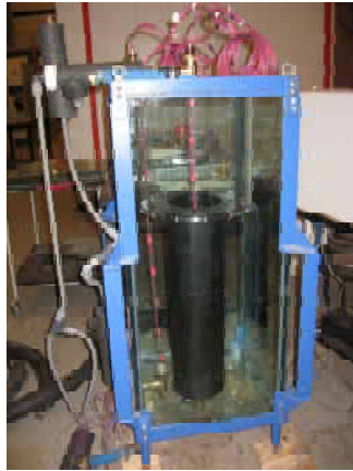
Fig. 1: Picture of the tank-in-tank heat store. The inner tank is for domestic hot water, whereas the outer tank is for water for space heating.
