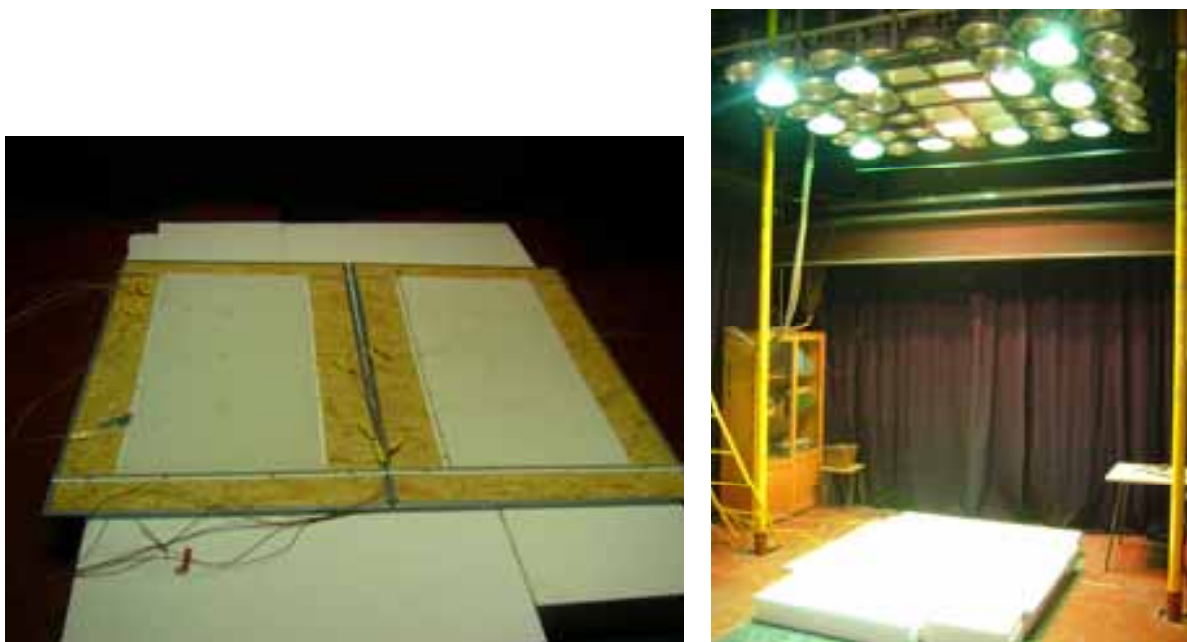
Fig. 6. Laboratory stand with test plates – charging process induced by radiation of solar simulator.
