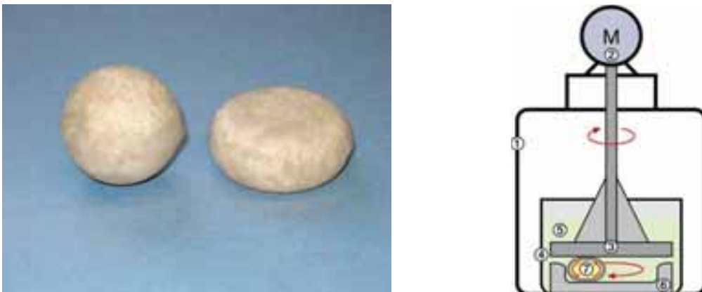
Fig.4: Non-deformed and deformed PCM-ball (left) and Set Up for churning test (1- furnace, 2 – motor and load, 3 – rotating disk, 4 – beaker, 5 – heat transfer fluid, 6 – support pad, 7 – PCM-ball)
