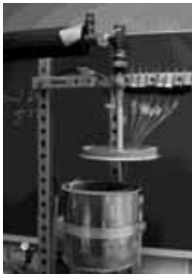
Fig. 4. Experimental setup for adsorption and desorption experiments (sorption store opened)
