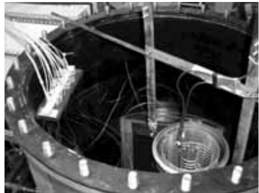
Fig. 6. Experimental setup for desorption experiments, sorption store from Fig. 4 and 5 including electric heating integrated into water store
