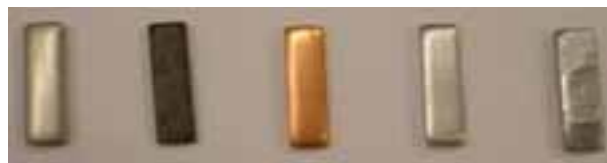
Fig. 1. Metal pieces used in the corrosion experiments. From left to right: stainless steel, laminated black steel, copper, aluminium, and galvanized steel
