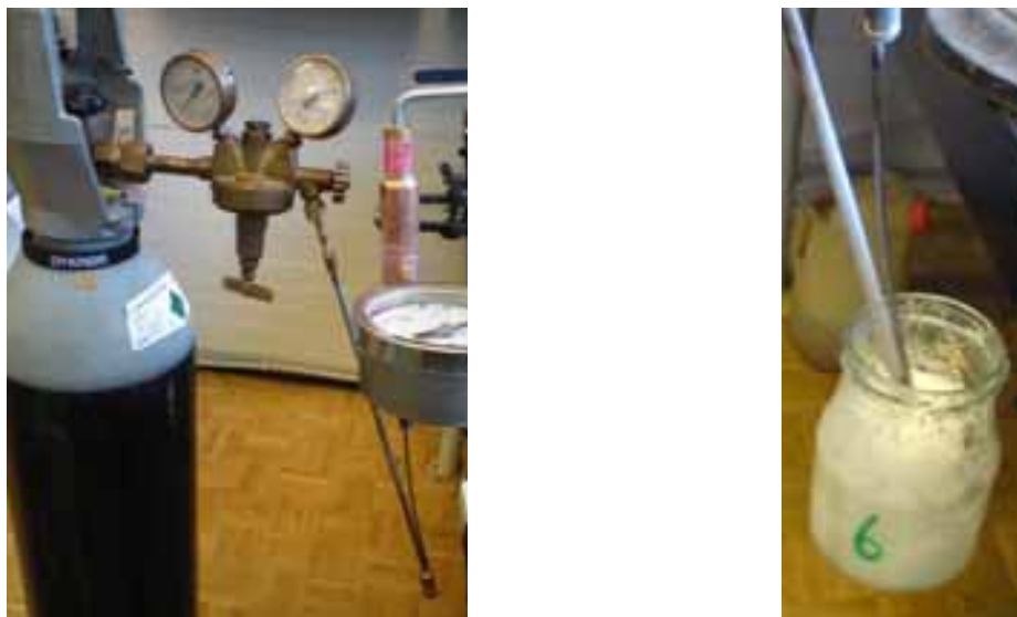
Fig. 2. Photos of the pressure container, the pressure reducing valve, the pipe system and the glass container.
