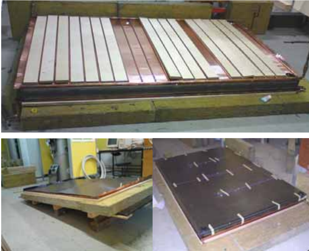
Fig. 8. Photos of the heat storage module.
