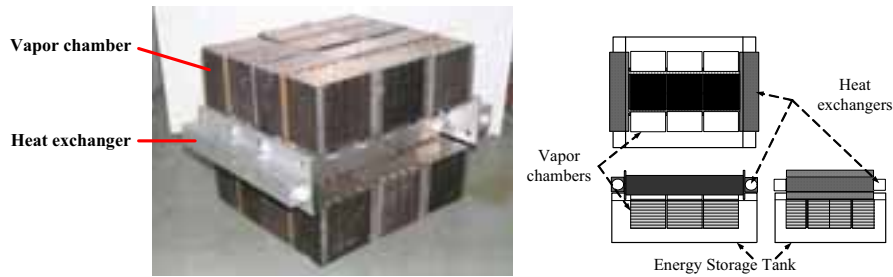
Fig. 1. The vapor chamber energy storage system.
