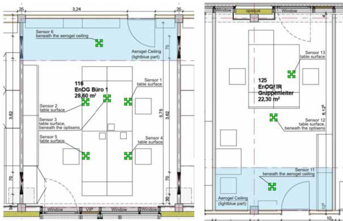
Fig. 7: Layout of a south-facing room (room 116, left) and north-facing room (room 125, right) equipped with additional illuminance sensors at the table surfaces and below the translucent (aerogel) part of the ceiling.
