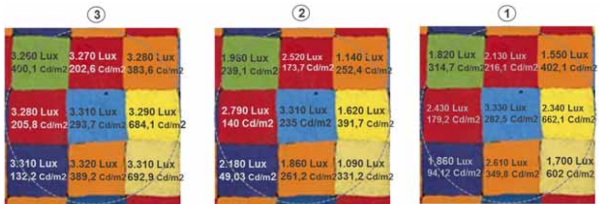
Fig. 8: Characterization of exhibition areas. Illuminances and luminances (Right to Left: 1 LEDs' Illuminant; 2 Halogen Incandescent Lamp; 3 Compact Fluorescent Lamp)
