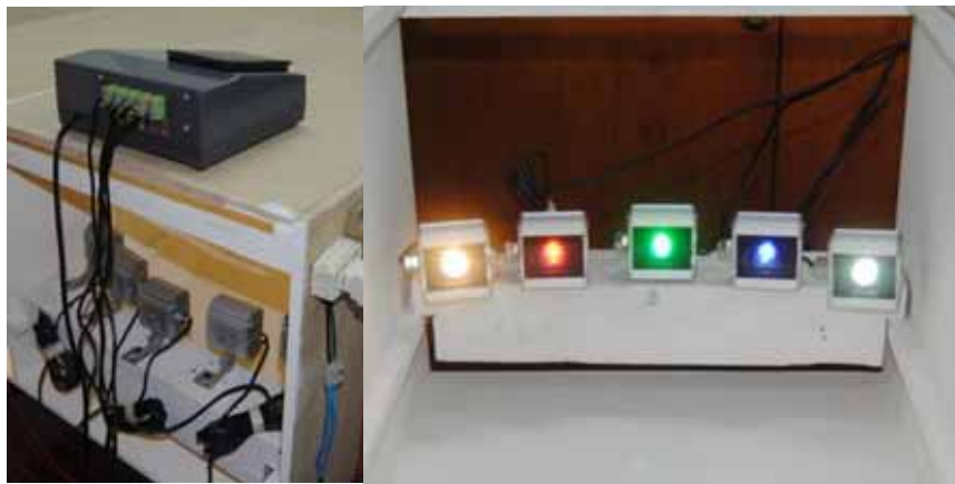
Fig. 6: LEDs' lamp adjustable device
