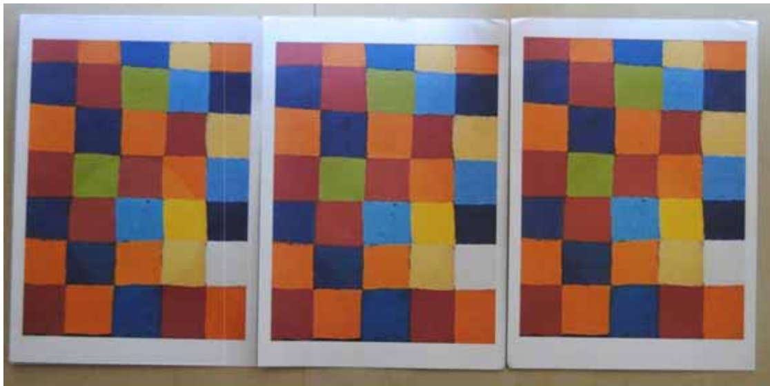
Fig. 9: Samples of M2 after the exposure to emissions (Right to Left: LEDs' Illuminant; Halogen Incandescent Lamp; Compact Fluorescent Lamp)
