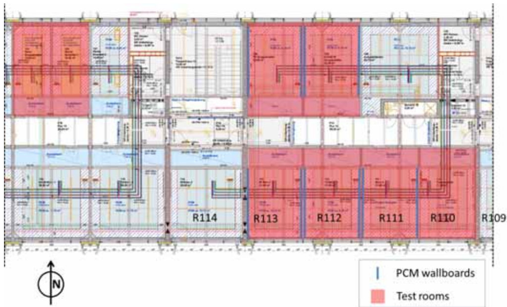
Figure 2: Part of the EEC second floor plan with the test-rooms and the positions of PCM wallboards highlighted
