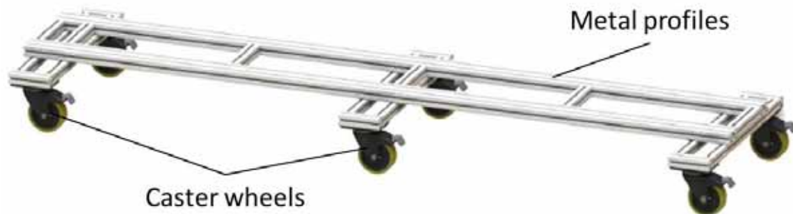
Fig. 7: Substructure for transportation of the prototype
