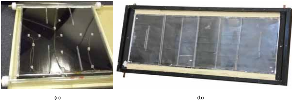
Fig. 1: The prototypes of the proposed PC+CNT solar collector: the first (a) and the second (b)
