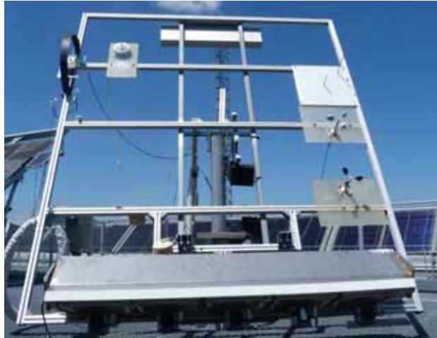
Figure 1: Picture of the whole solar tracker for collector testing.
