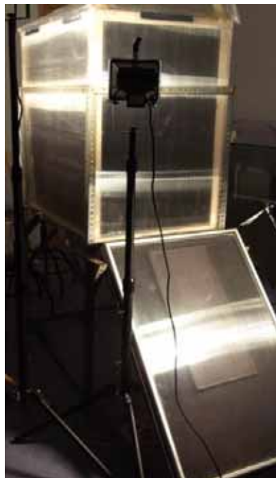
Fig.3: Irradiating the solar dryer by the power lamps during the experiment.
