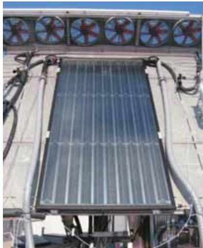
Fig. 2: Real geometry placed on the tracker for measurement of collector efficiency
