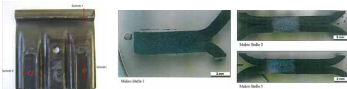
Fig. 13: Left: Sample after a corrosion test at FQZ Oderbrücke gGmbH. The red lines indicate the cuts where grinding marks were prepared and visually examined for corrosion, right: prepared grinding marks.
