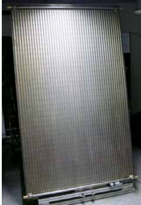
Fig. 3: 2-m 2 steel absorber with harp design (back side) produced by pressing half-shells and a downstream welding process without coating.
