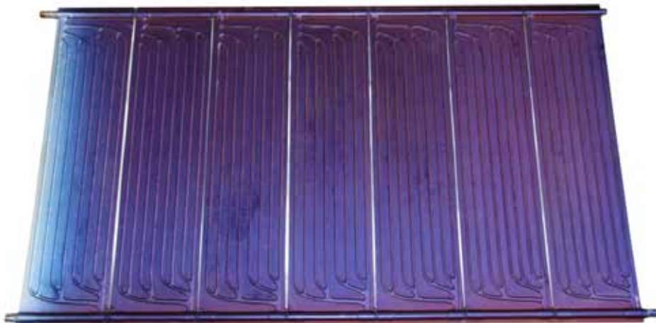
Fig. 4: 2-m 2 modular steel absorber with FracTherm ® channel design produced by partial cold roll bonding and hydroforming with a spectrally selective coating.
