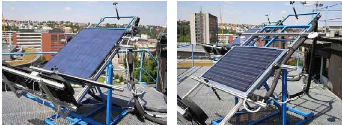
Fig. 3: Tested solar PVT absorbers: state-of-art (left), developed CTU prototype (right)
