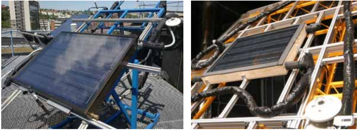
Fig. 5: Glazed nonselective PVT collector at outdoor testing, glazed selective PVT collector at indoor testing
