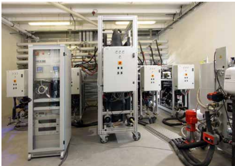
Fig. 1: Picture of the absorption chiller connected to the INES test bench
