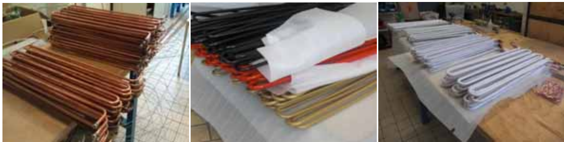
Fig. 2: Bended copper tubes; before powder coating (left), after powder coating (middle) and with Tencel® sleeves (right)
