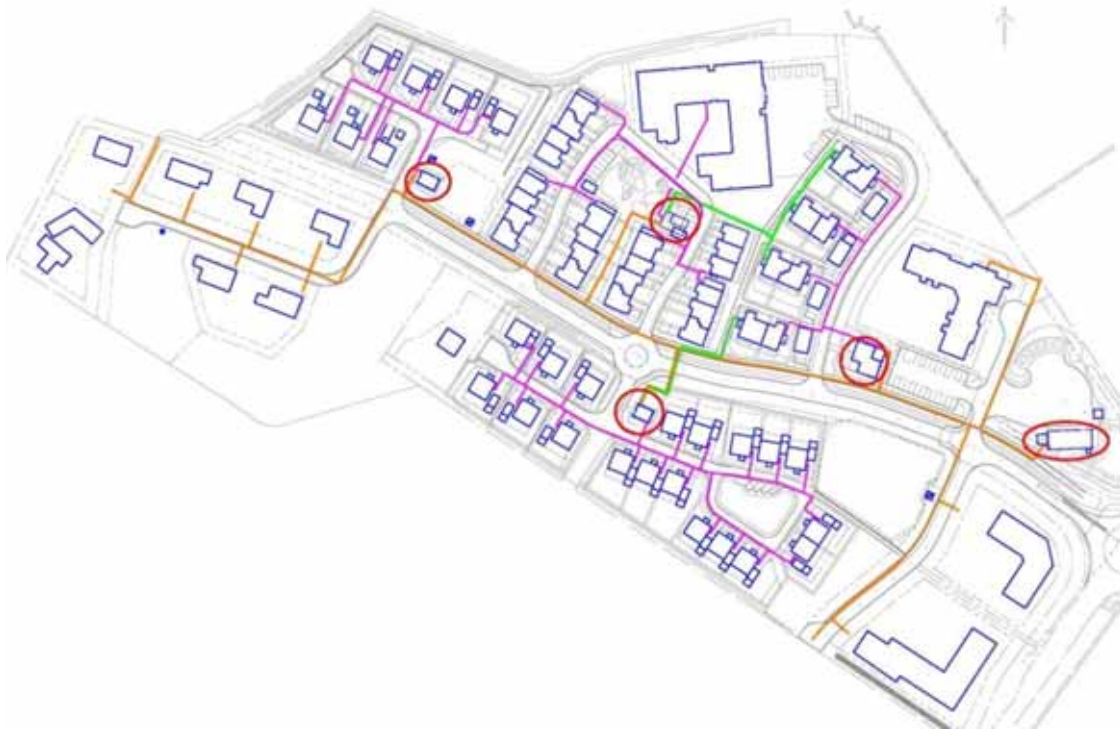
Fig. 6: Building area with central heating plant (right), four sub-stations (red), primary (brown) and secondary (violet) heat distribution, as well as the distribution system for solar heat (green) between the 4 multifamily buildings and sub-stations 1 (at bottom with 19 single family buildings) and 3 (top middle with 22 units in terrace buildings and the nursing home for elderly people). Sub-station 2 is in top left (see also Fig. 11). The 6-7 small buildings shown on the far left and 3 large buildings nearby the heating plant are not yet built.
