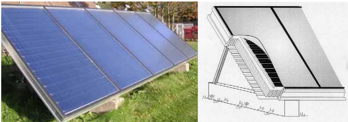
Fig 3. Photo and skematic sketch of solar collector with foil from ARCON Solar A/S tested at the Technical University of Denmark in 2007.
