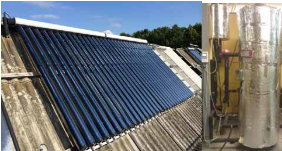
Figure 1b. Lab system at DTU: Photo of the ETC solar collector in winter with snow, storage tank, controller, auxiliary heater and drain back vessel.
